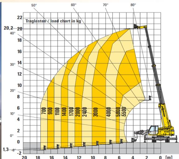
**Spécifications:** Poids engin: 23600 Kg Charge maximale: 8000 Kg
